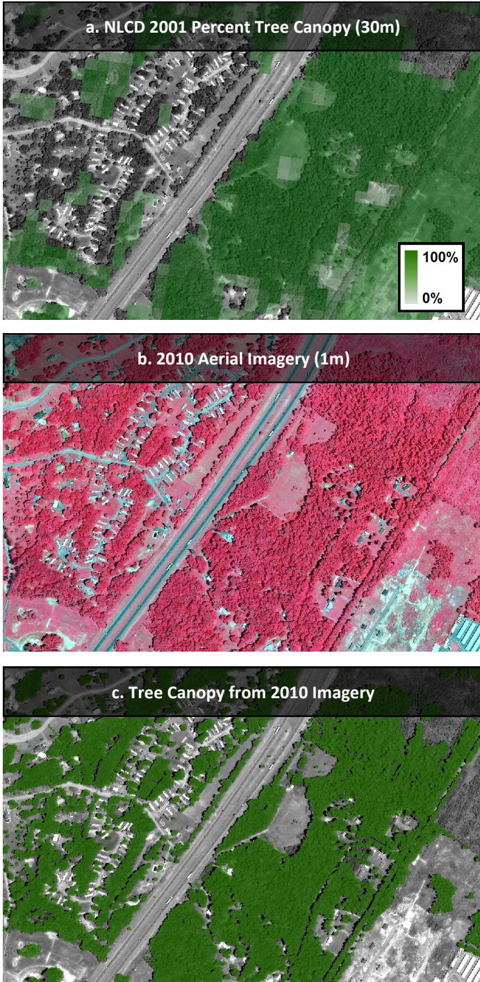
Figure 3: Comparison of NLCD 2001 (a) to high-resolution imagery (b) and tree canopy (c) derived for this study.
